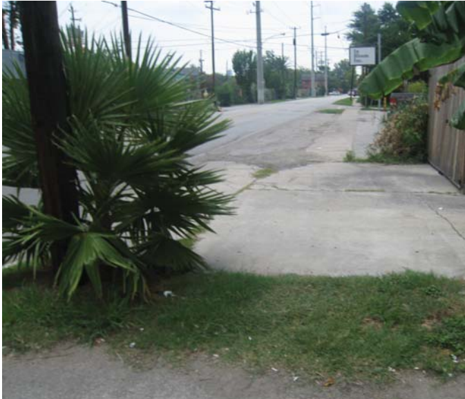
Photo 8-23, Segment 48A Fairview between Converse and Crocker Sidewalk is missing. Vegetation growth in the sidewalk which makes it difficult for pedestrians to use the sidewalk.
